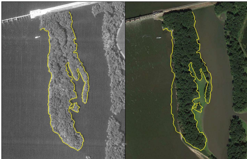
Figure 2. Example of bankline erosion and forested island loss between the main channel and Swift Slough in upper Pool 11, 1994–2013. Yellow line depicts extent of tree canopy in 1994.
